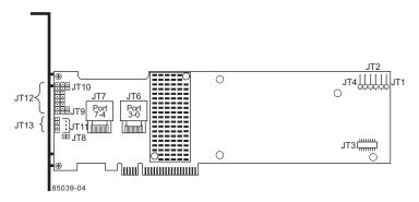
Note: JT1, JT2, and JT4 are behind the LSIiBBU07 when the iBBU is installed, but they are still accessible.
